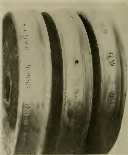
FIG. 1. EXCESSIVE BRAKE BURNING AND COMBY TREAD.
